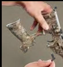
Remove the safety spring and detent, and pull out the safety selector.
