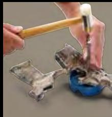
Use a punch to drive out the trigger pin.
